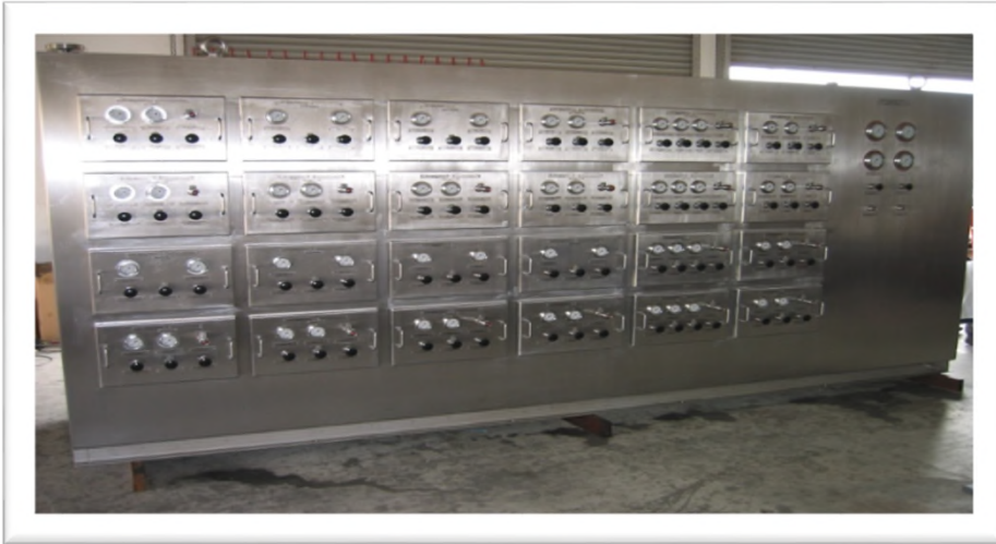
WHCP Front View (14 Oil Wells, 6 Water Injection Wells and 4 Gas Wells)
