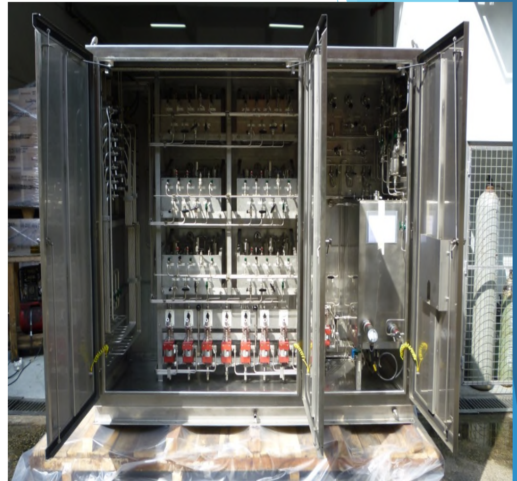
Six Wells Completion Modules retractable type wellhead control panel front & rear view.
