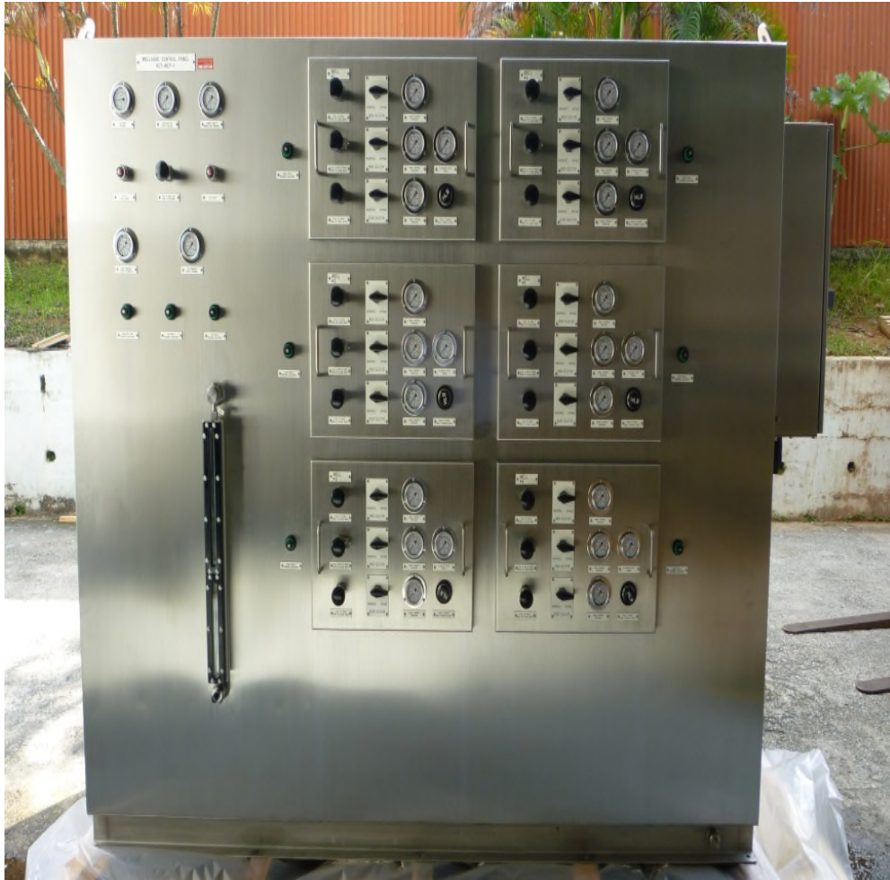
Six Wells Completion Modules retractable type wellhead control panel front & rear view.
