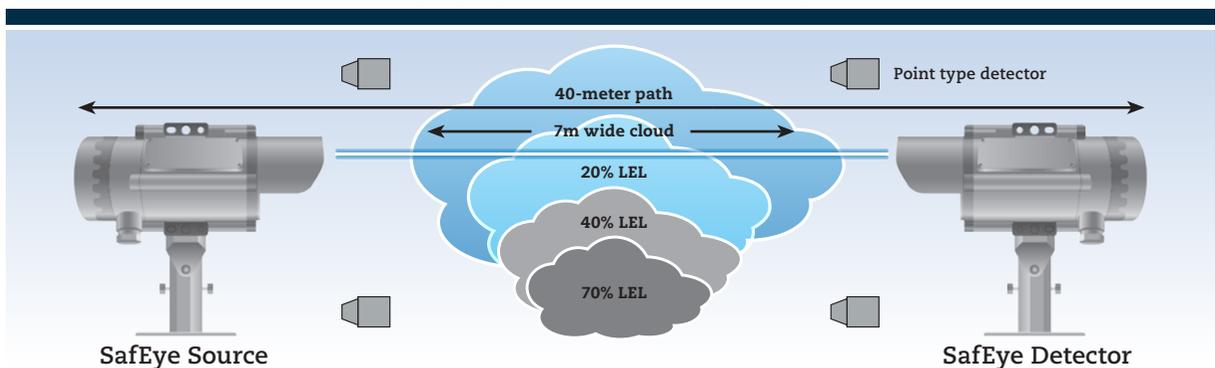
This scenario shows how the matrix of point type detectors can miss a leak or eventually only see diluted gas levels whereas SafEye 900 Open-Path will, in this case, measure 20% LEL x 7m = 1.4 LEL.m - well above 1 LEL.m alarm level
