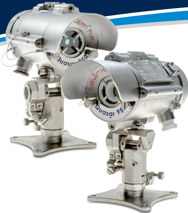
The latest SafEye Quasar open path UV detection technology includes the 950 and the 960 series. The Quasar 950 models detect toxic Hydrogen Sulfide gas and the Quasar 960 models detect toxic Ammonia gas, both with path lengths of up to 200ft (60m). The Quasar 950 and 960 models can be tailored to protect your personnel and high-risk installation. Reliability is key and is assured with SIL2.
