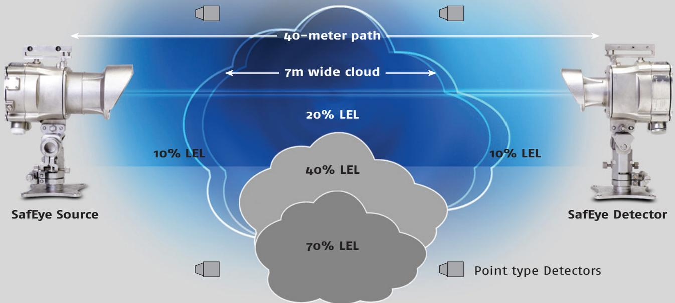
*This scenario shows how the matrix of point type detectors can miss a leak or eventually only see diluted gas levels whereas SafEye 700S Open-Path will, in this case, measure 20% LEL x 7 m = 1.4 LEL.m - well above 1 LEL.m alarm level*
