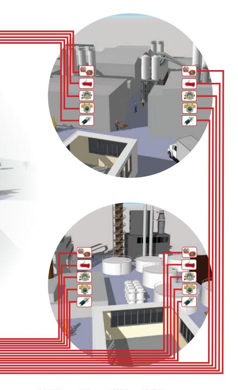
A combined approach could be used, for example to expand an existing system. New Inputs and Outputs required due to an expansion of a production area could be connected to a remote Touchpoint Pro unit, while the existing system and cabling are wired directly to the Touchpoint Pro central controller.
